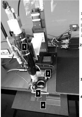
1 Microscope module for *in situ* process control (image and video aquisition)
